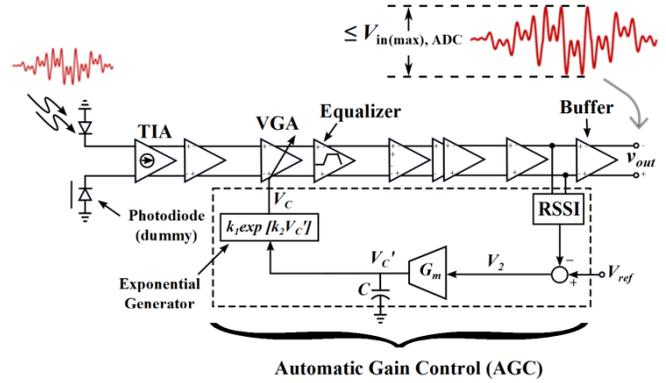
Figure 7: Example of an analog optical receiver architecture for software defined optical communication.
