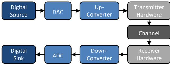
Figure 2: High-level signal chain for a software defined communication link.
