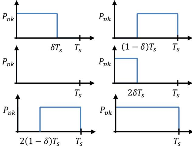
Figure 13: Symbol sets for dimming modulation schemes  $\delta$ -VPPM (top),  $\delta$ -RTZ (center), and  $\delta$ -RTZ-I (bottom).
