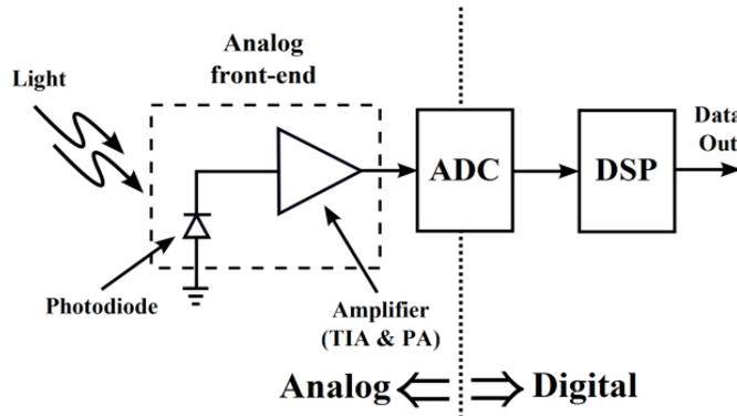
Figure 4: SDVLC Optical receiver front-end.
