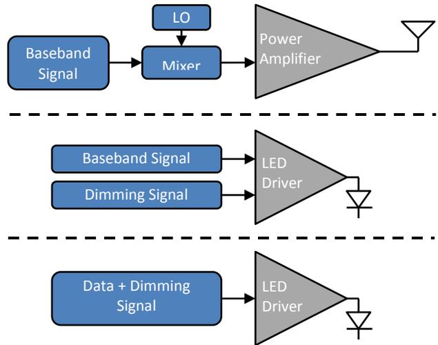
Figure 3: Signal chains for an SDR transmitter (top), an SDVLC transmitter with dimming and data as separate inputs (center), and an SDVLC transmitter with a single input with combined data and dimming signal (bottom).
