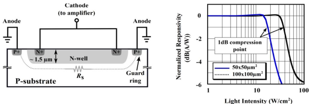
Figure 5: Non-linearity in Si photodiodes: (left) a Si N-well/P-substrate photodiode showing bulk series resistance, (right) simulated responsivity vs. input power showing the effect of area on photodiode non-linearity.
