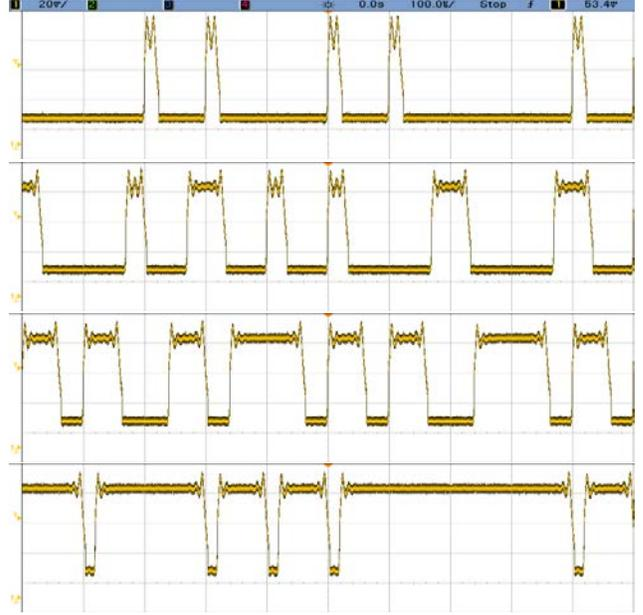
Figure 14: Received electrical signal from the optical receiver for 0.1-RTZ, 0.3-VPPM, 0.6-VPPM, and 0.9-RTZ-I.
