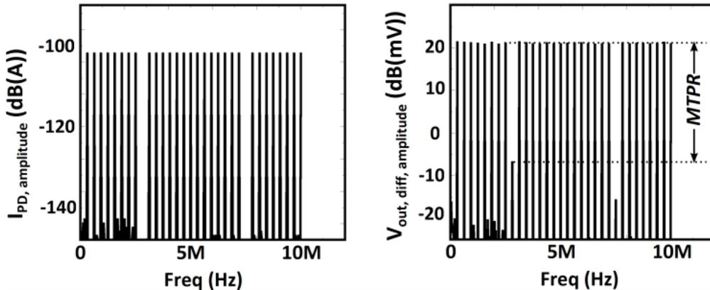
Figure 8: Simulation results for MCM: (left) 30-subcarriers with 2-missing tones at the input (PAR=4.86dB), (right) Spectral-regrowth in missing sub-carrier location at the output (MTPR=28dBc for  $V_{out,p-p} = 200\text{mV}$ ).
