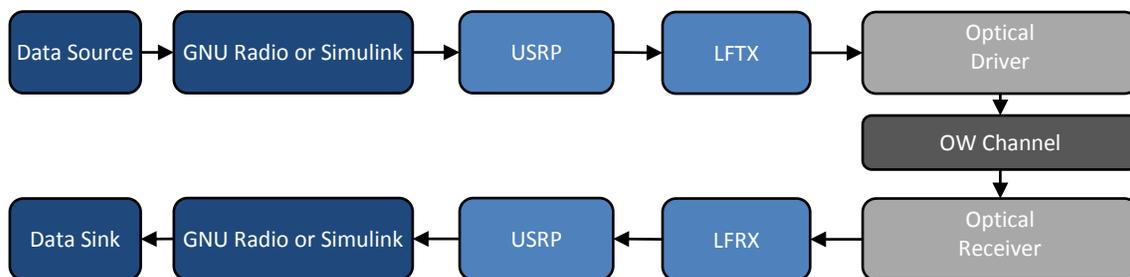
Figure 9: Signal chain for the SDVLC implementation.
